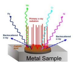
test on the material at any time in merely seconds. XRF works by exposing the material to a flux of x-rays. The atoms then absorb the
