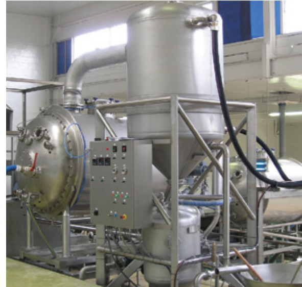
Turnkey production system for vacuum cooking of jam installed in 2009 consisting of 2x2500 L (2x600 gallons) HPTs and a condensing system with aroma recovery.
