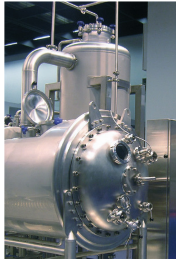
Turnkey production system for vacuum cooking of jam installed in 2009 consisting of 2x2500 L (2x600 gallons) HPTs and a condensing system with aroma recovery.
