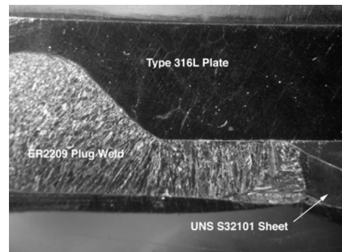
Figure 3-Macrosection of Plug Weld
